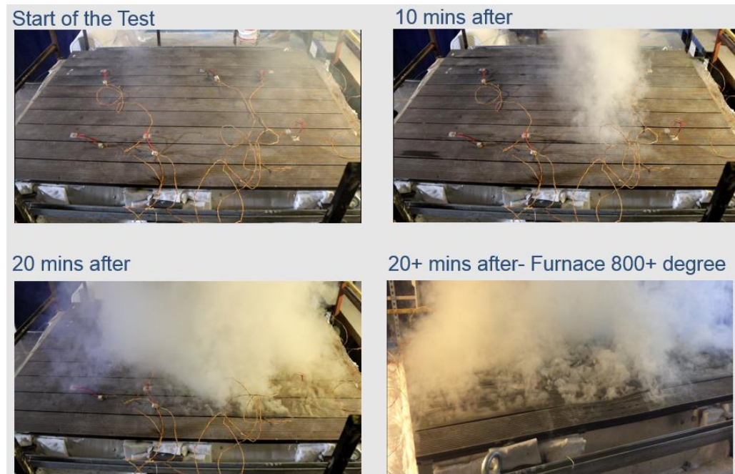
Photos showing the test balcony mounted on the furnace at various stages
