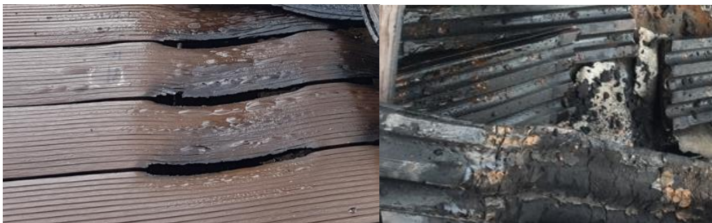
Photos showing the top side and underside of the boards following the test.
