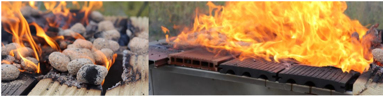
Photos showing the decking during test. From left to right, Class A. class B, 2x class C , timber .
