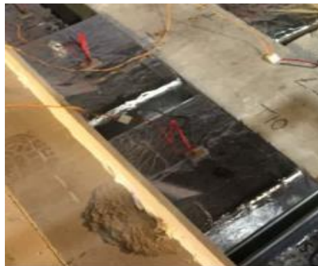
Fig.4 Testing of StubGuard™ at Exova – note sensor monitoring top surface temperature
